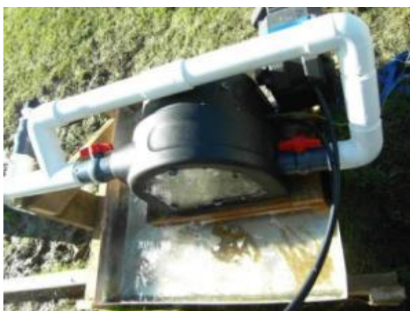
PowerSpout PLT200 running at 1500W
